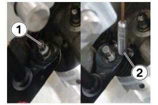
23. When the valve stem and keepers are exposed (1), the keepers can be removed with a magnet (2).
