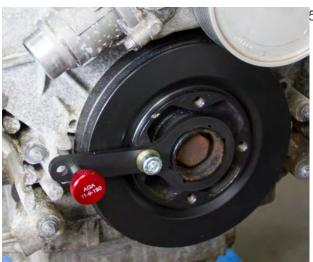
50. When the crankshaft is positioned correctly, install AGA-11-8-570 Crank holder and AGA-11-9-190 Pin, or BMW equivalent tools.
