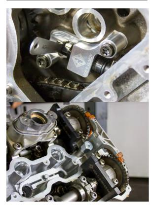
44. When the crankshaft is positioned correctly, install AGA-11-8-570 Crank holder and AGA-11-9-190 Pin, or BMW equivalent tools.
